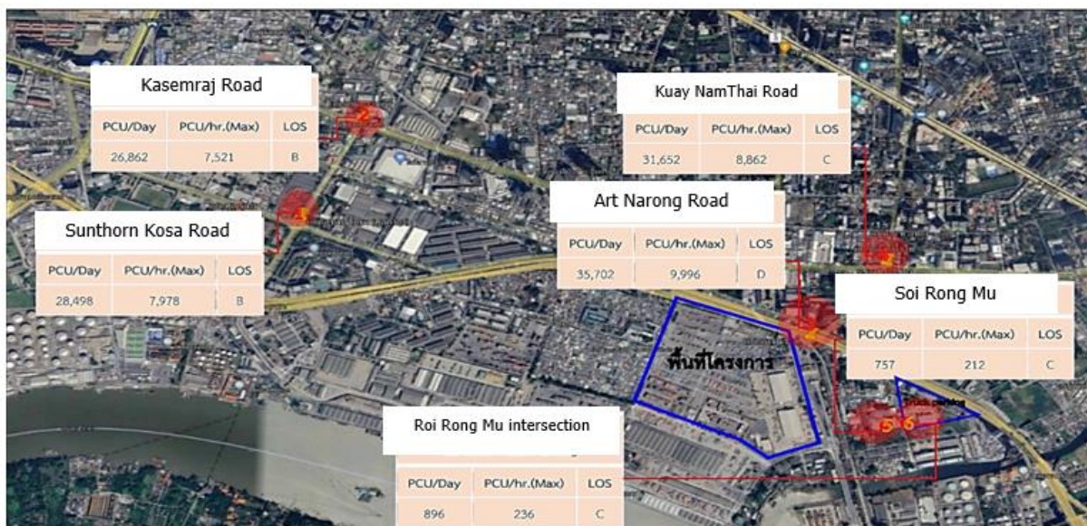
Figure 3: Traffic volume in MC and TMC (intersections) outside Bangkok Port (Surveyed on September 2024)
