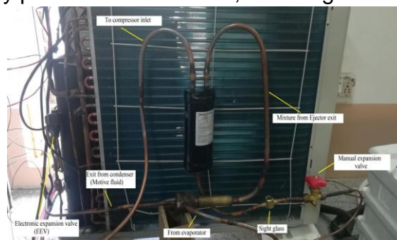
Fig. 7 Ejector split air conditioner (ESAC)
