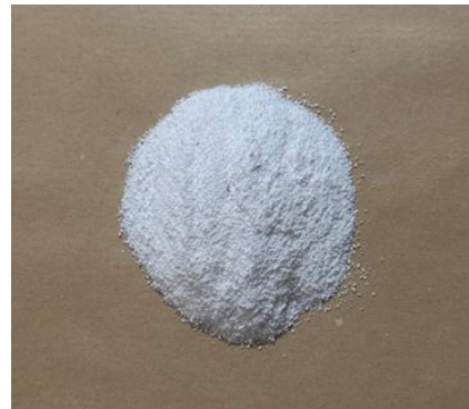
Fig 11: \beta -TCP nano-powder produced following hydrothermal treatment and calcination
