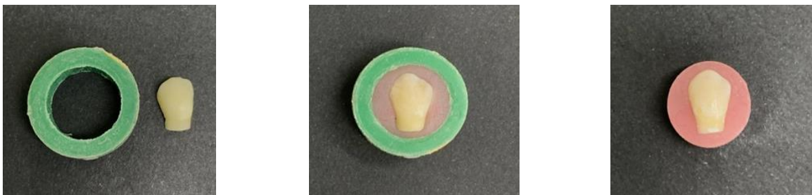
Fig 6: Steps of teeth mounting in the acrylic resin
