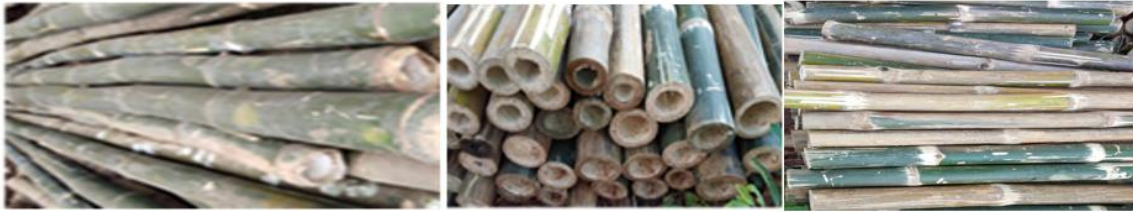
(e) Harvested Matured bamboo (f) Cut with one -node (g) Cut with two-nodes
