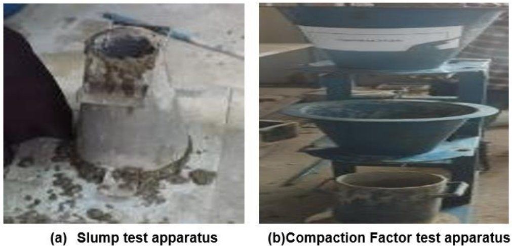
Figure 3: Apparatus used for workability of concrete
