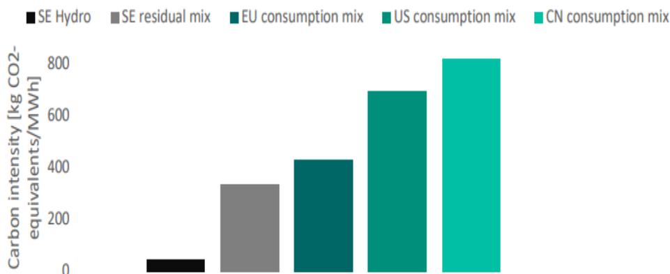
**Figure 10: Carbon Intensity of Different Electricity Mixes used in the Sensitivity Analysis**
