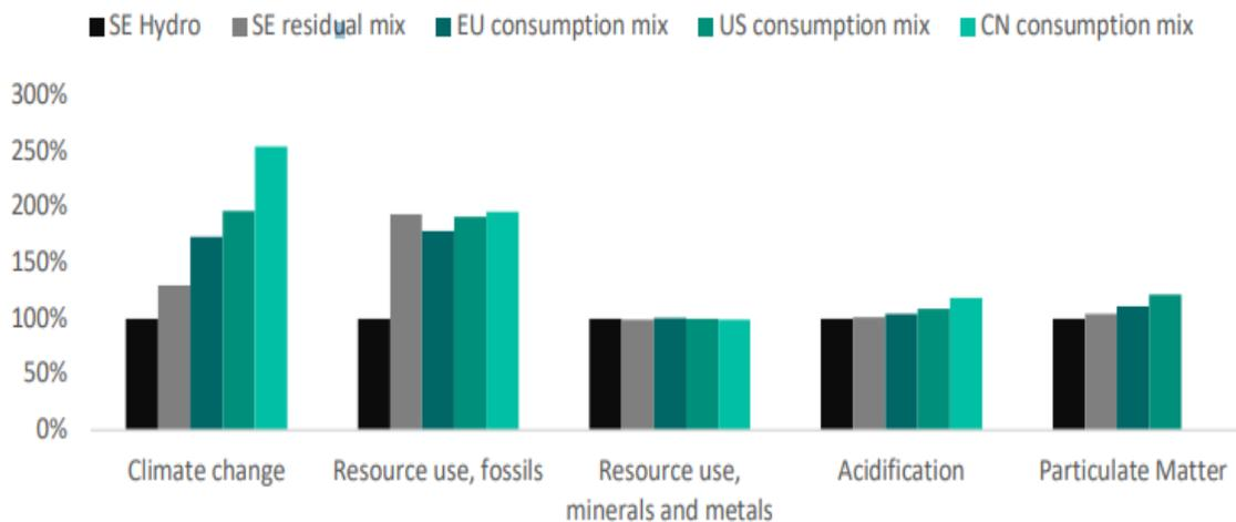
**Figure 11: Sensitivity analysis for the carbon intensity in the electricity mix used in battery cell production impact on the characterised result of climate change, fossil resource use and water scarcity results**
