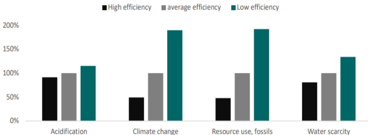
**Figure 13: Sensitivity analysis on the round-trip efficiency of the battery pack influence on characterised acidification, climate change, fossil resource use and water scarcity results**
