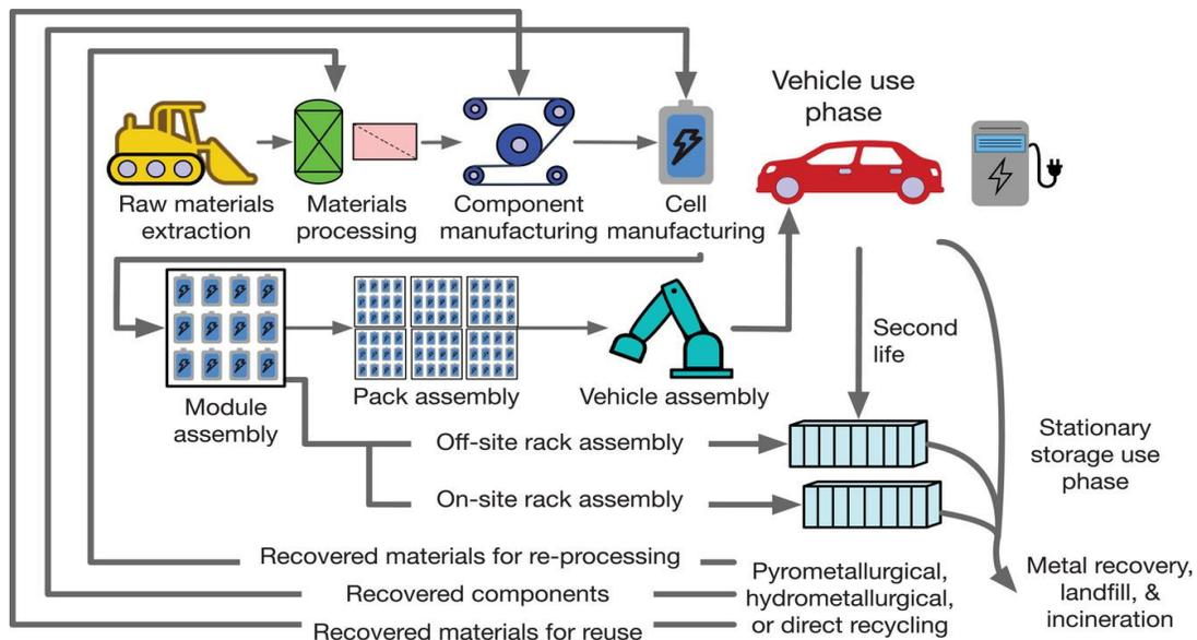
**Figure 1: Major life-cycle Stages for Vehicles and Stationary Batteries**
