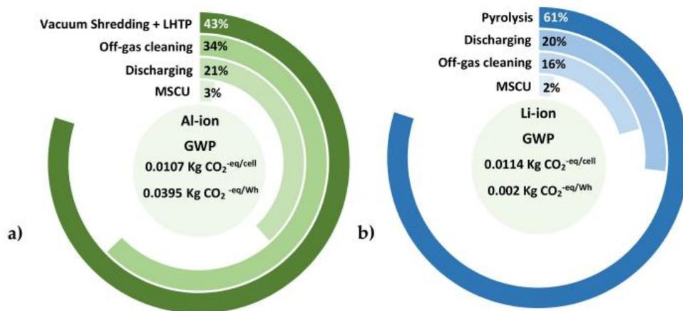
**Figure 9: Comparison of the GWP Contribution by the Al-ion's (a) & Li-ion's (b) Recycling Processes**
