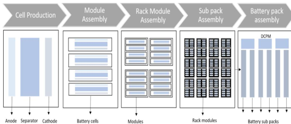
**Figure 3: Production Stages from Battery Cell to Battery Pack**
