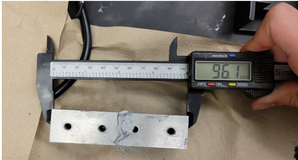
Figure 15.1: Measuring the thickness using calipers
