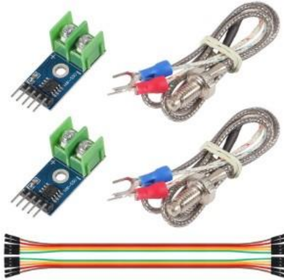
Figure 14: shows the K-Type of thermocouple selected for this experiment
