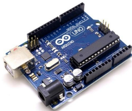
Figure V: Arduino UNO R3 Development Board with on board chip
