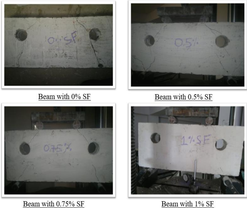
Fig 8: Failure of deep beam having opening at position A
