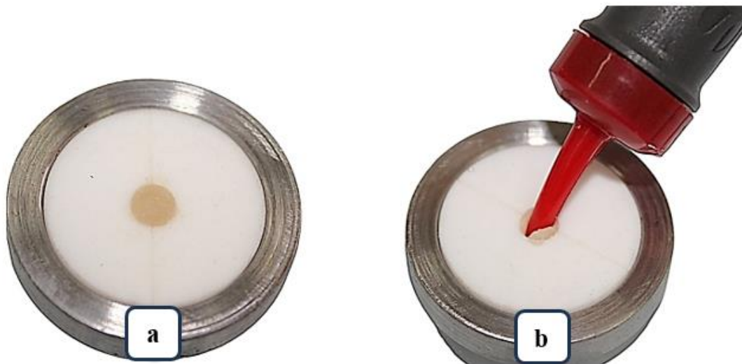
Figure 4: a & b SureFil and Surefil one inserted in one increment of 4 mm thickness
