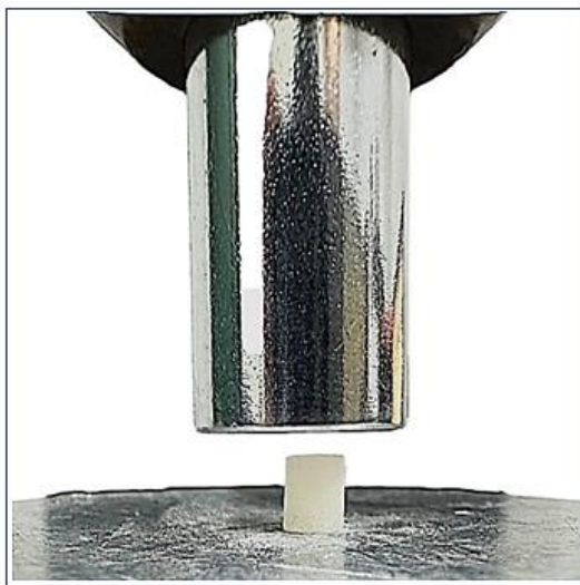
Figure 7: Compressive load along the long axis of the specimen
