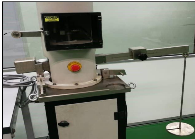
Fig.2: View of Four Ball Tester machine is used(KOEHLER K93190-M)
