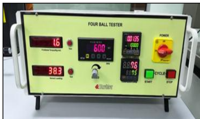
Fig.3: Duration of testing is set at 60 minutes for each test.
