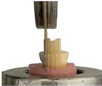
Figure 9: Sectioning in mesio-distal direction
