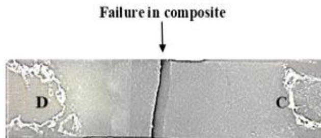
Figure 16: Showing M failure. D: dentin, C: Composite. At 50x Magnification
