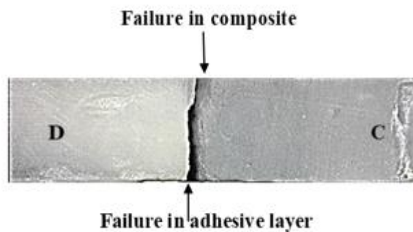
Figure 16: Showing M failure. D: dentin, C: Composite. At 50x Magnification
