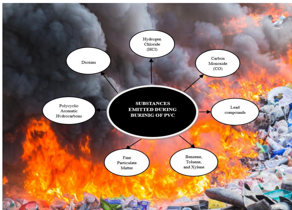
Figure 1: Substances emitted during the burning of PVC waste
