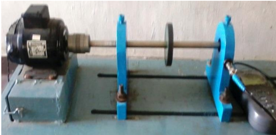
Figure 1: Experimental set up of rotor kit with FFT analyzer.
