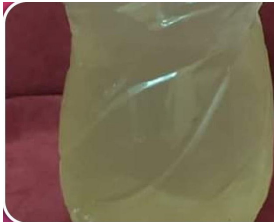
Fig.5. A photographic to a sample of wastewater from a Bilbeis drain with turbidity 52.20 NTU
