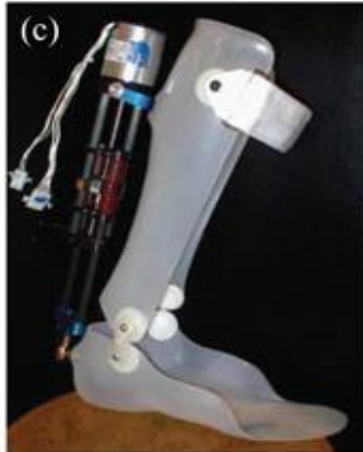
Fig 3: The MIT active AFO powered by a series elastic actuator. From [27, 30, 31, 35]. This figure is reproduced from Shorter, Xia [2] with permission
