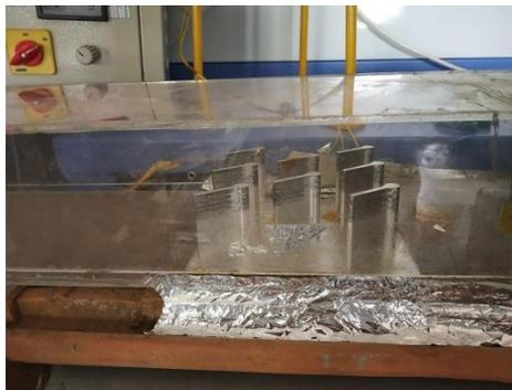
**Figure 3. Heat sink in duct**
