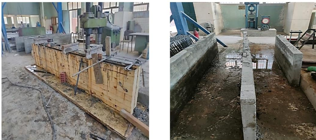
Fig.2: Preparing of casting and curing of the tested beams.
