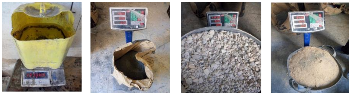
Fig.1: Weigh the components of the concrete mix.
