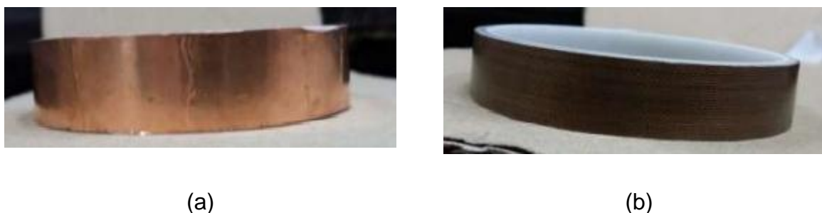
Figure 4: (a) Copper tape as electrode barrier and (b) Teflon tape as a dielectric barrier.
