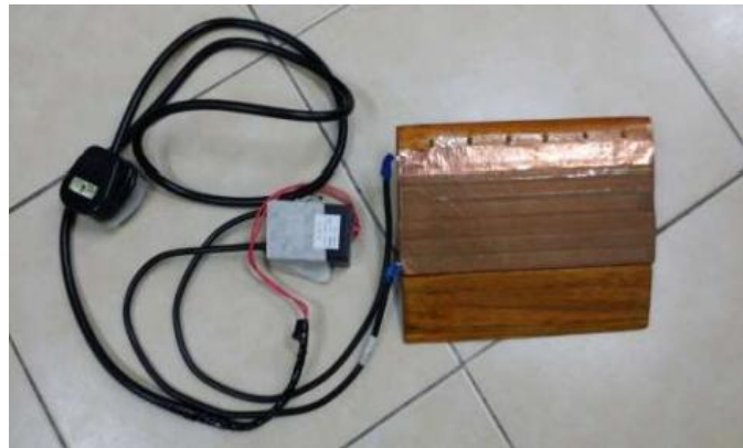
Figure 5: Final attachment of plasma actuator on the airfoil
