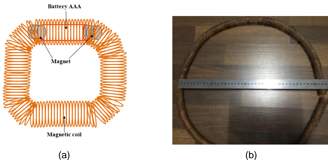
Figure 4: The diagram of the magnetic coil for weight and time testing in diameter distance illustrated in (a) schematic diagram, (b) prototype
