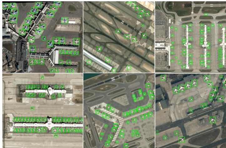
Fig 5: Detection results by the QATM-KCNN model (in green)
