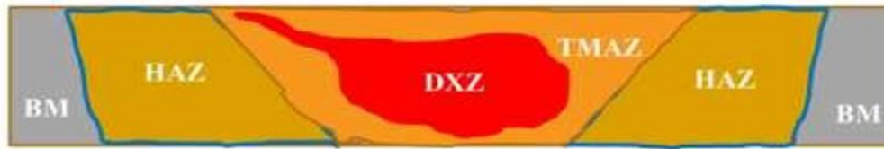
Figure 2: Illustrative map of FSW joint zones [2]
