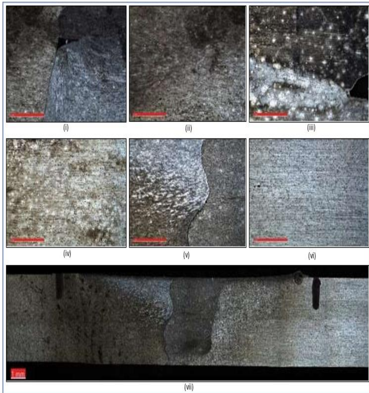
Figure 6: Optical microscopy of (i) NZ of AA2024 (ii) BM of AA2024 (iii) NZ of AA7075 (iv) BM of AA7075 (v) NZ of AA2024/7075 (vi) BM of AA2024/7075 (vii) Macroscopic view of AA2024/7075
