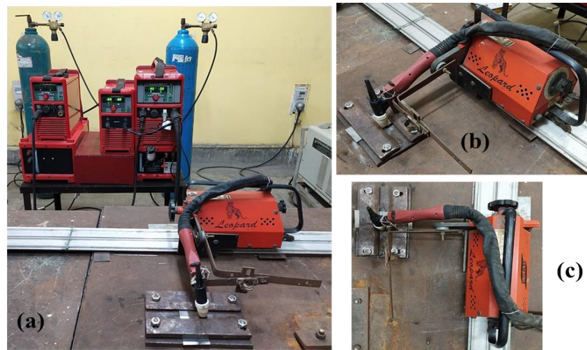
Figure 1: In house developed plasma arc welding experimental setup
